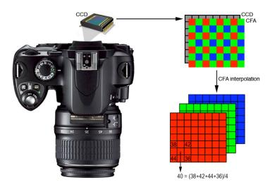
**Figure 1:** A color filter array (CFA) overlaid onto a CCD sensor. Each CCD element records a limited range of wavelengths, corresponding to either red (gray), green (light gray), or blue (dark gray). A full three channel RGB color image is created by interpolating the missing color pixels by, for example, averaging the recorded values.
