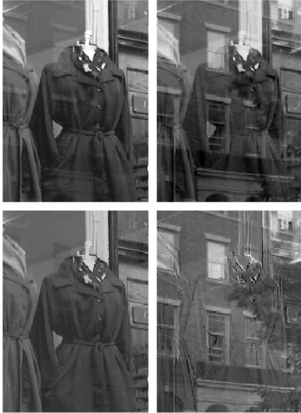
Figure 11: Shown along the top row are the pair of images photographed through a linear polarizer at orthogonal orientations, and shown along the bottom row are the separated components.
