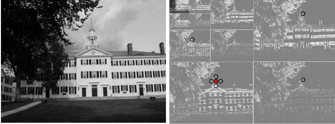
Figure 2.8: A natural image (left) and the magnitudes of its three-scale QMF pyramid decomposition (right). Note the correlation between magnitudes of neighboring coefficients, as highlighted in the right panel and corresponding to the fixed neighborhood set used in Equation 2.19.
