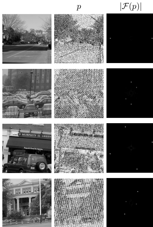
Fig. 7. Shown are four images affine transformed by random amounts. Shown in the middle column are the estimated probability maps ( p ) that embody the spatial correlations in the image. The Fourier transform of each map is shown in the right-most column. Note that these images yield periodic maps.
