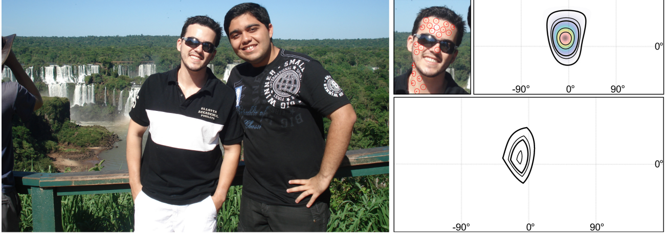
Figure 1. An analyst specifies 3-D surface normals (red probes on the face) from which the 3-D light direction is estimated (visualized as a probability in azimuth/elevation in the upper right panel). Multiple such constraints are combined to determine if lighting in the entire image is consistent, as in this example (lower right panel).
