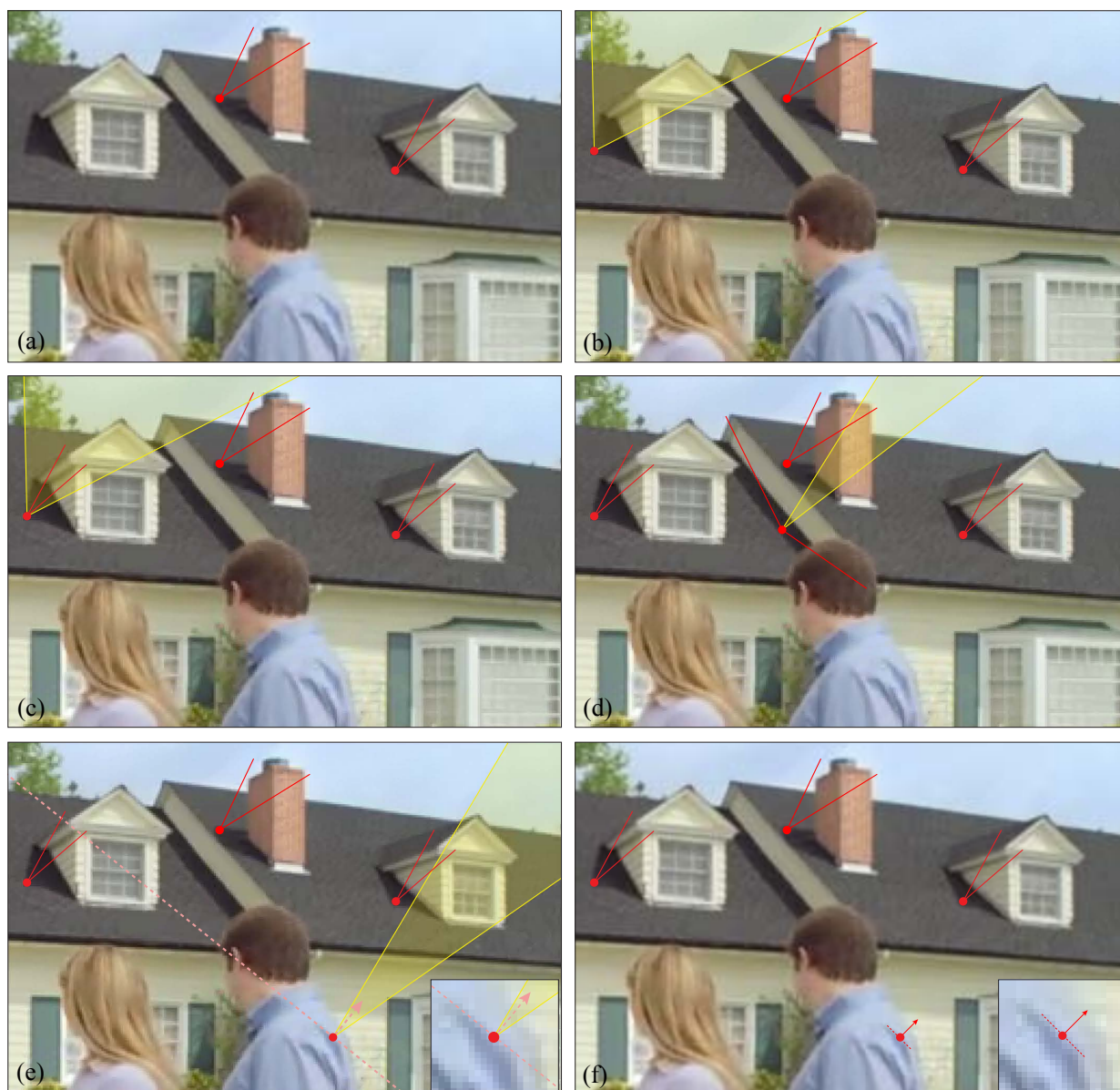
Fig. 5. A user interface for specifying shadow constraints: (a) two cast shadows are manually selected on the roof; (b-c) an analyst specifies a point on a cast shadow (red dot) and automatically the range of plausible light directions is rendered (yellow wedge). Specification of a constraint (c) reduces the width of the wedge to conform to the object casting the shadow (red lines); (d) a constraint may be ignored if the yellow wedge is too narrow to reliably encompass the object which cast the shadow; (e-f) an analyst specifies a point on an attached shadow (red dot) and the orientation and direction of the shadow terminator is automatically suggested by computing the image gradient (pink dotted line and arrow) after which an analyst can accept or adjust the constraint.
