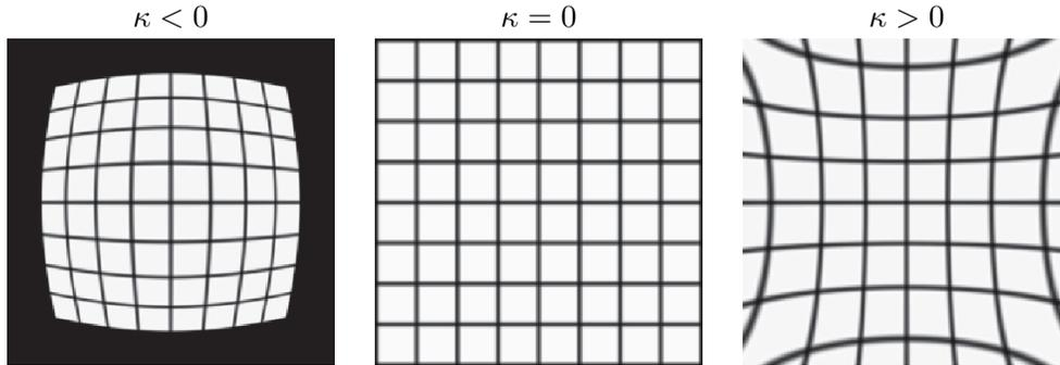
**Figure 9:** Radially symmetric lens distortion, Equation (32).
